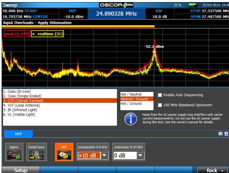
To clear the error, apply just enough attenuation until the input overload warning is no longer displayed. If the signals are still present after the attenuation is applied, they should be considered actual threats.
