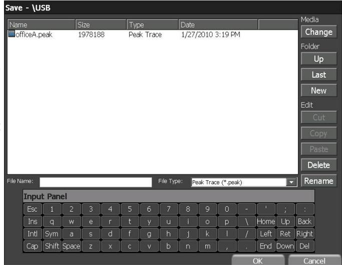
At this point walk into Office B to collect a Peak Trace using the same steps as above. It is important to clear the Peak Trace in Office B to ensure that no signal levels from Office A corrupt the spectrum of Office B. Save the trace in Office B using the steps given above.
