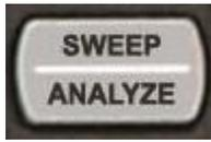
Press **Sweep/Analyze** to enter Analyze Mode. In this example, the wireless microphone was demodulated and "listened" to using the audio demod.
