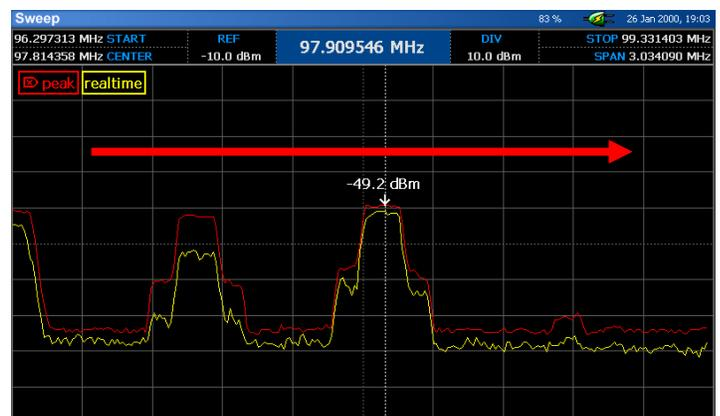
Position the cursor on the desired signal by tapping the signal with your finger or the stylus.
