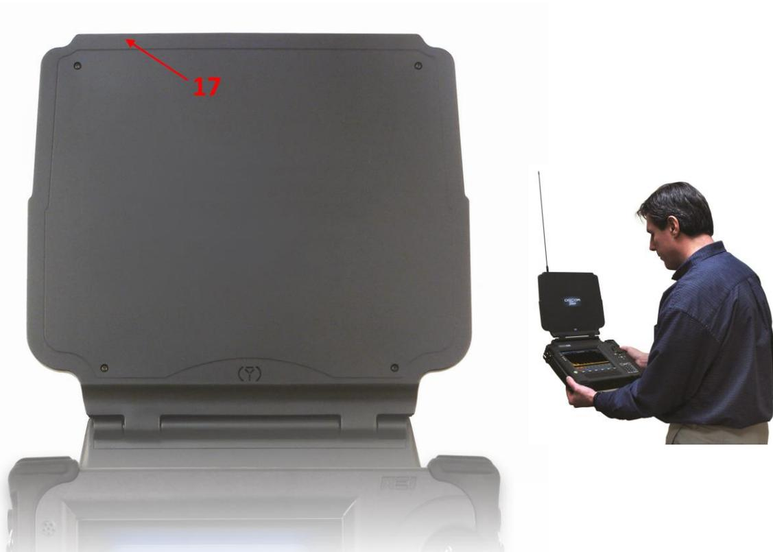
17. **Whip Antenna Connector** – for connecting the whip antenna accessory to improve low frequency reception
