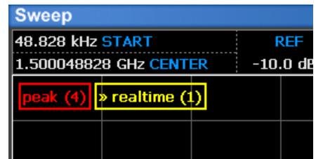
Notice the Sweep Counts displayed in the top left corner of the spectral display. This keeps track of how many sweeps are included in each displayed trace. The sweep count for each trace is displayed beside the trace name.
