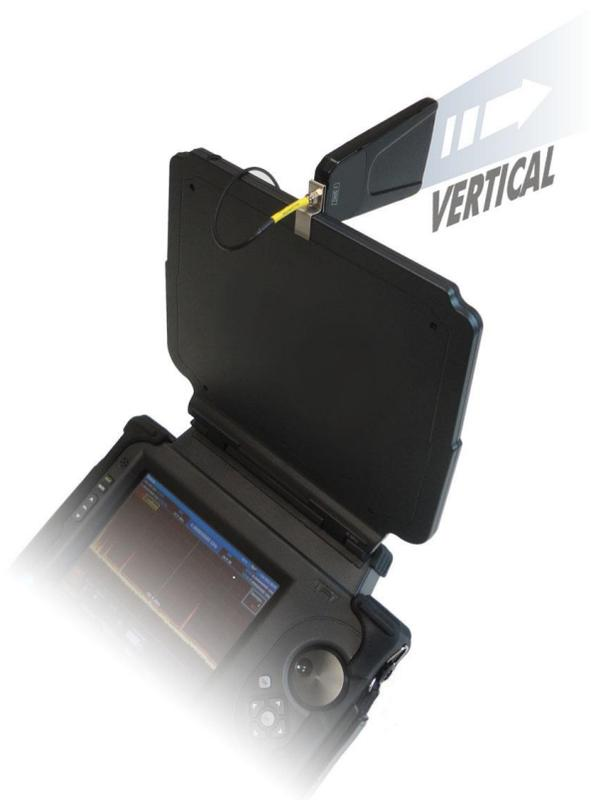
18. **Directional Antenna \*** –Clip the included Vivaldi directional antenna to the antenna panel and connect to the 0 – 8 GHz Auxiliary input on the back of the OSCOR unit for improved directivity in the 1.5 GHz to 8 GHz range.
