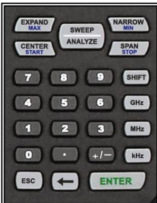
Type in a known FM radio station from the numeric keypad. (95.5 MHz is shown in this example; You should use a known station in your area.)
