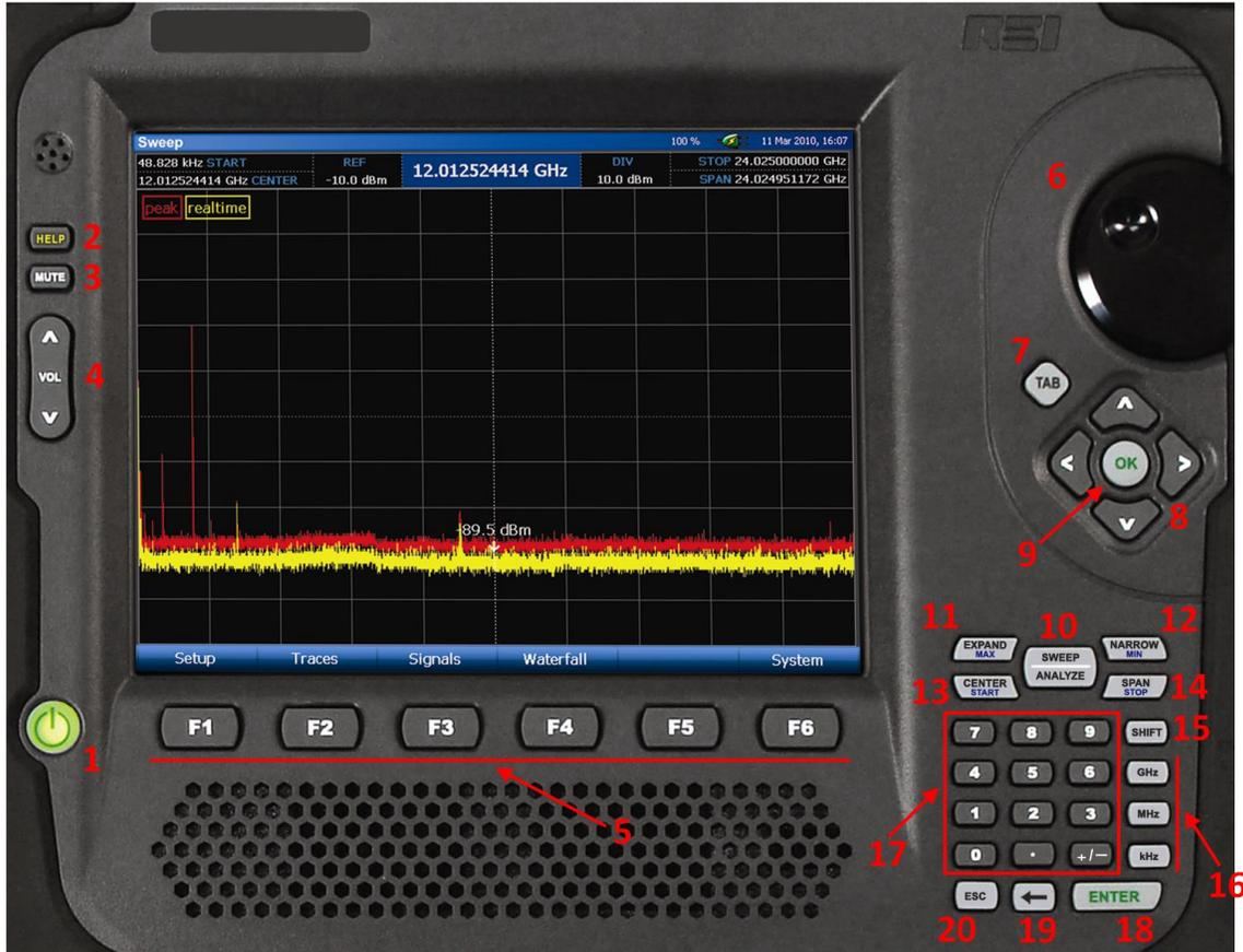
1. **POWER** – turns the unit off and on. Press and hold the power button until the unit shuts off to do a firmware reset. As the unit powers on, the power button will display various patterns of solid and blinking colors to indicate successful initialization and self-test. This is a list of the various colors the power button will display during operation and what each color indicates:
